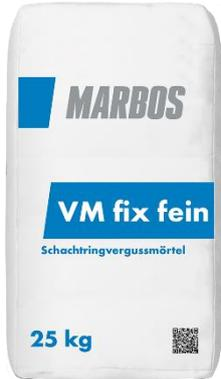
For play-free, extremely fast loadable and force-locking grouting and underfilling of joints between shaft frame and substructure, machine frames, crane rails, bridge bearings, high rack supports, concrete finished parts, anchors, etc.
